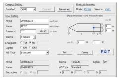
Select AIS type. (Standard is for vessel; AtoN is for buoy; Older AIS is for vessel with older chartplotter it can't receive Name of vessel.)
